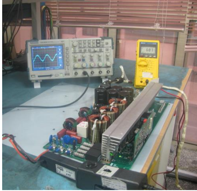
Fig. 6. The designed three phase rectifier
